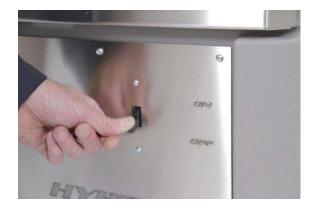
When the vacuum has new filters in it and it has no hose attached the motor is running with little restriction. And will run at approximately 15 Amps.
